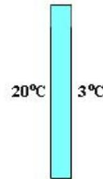
$$\frac{\Delta Q'}{\Delta t} = k_V A \frac{(30 - 3)}{\Delta X} = 11,3 \frac{\text{cal}}{\text{s}},$$
