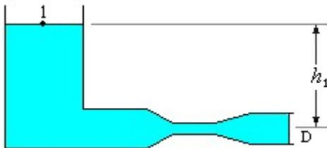
$$p_1 + \rho g h_1 + \frac{1}{2} \rho v_1^2 = p_2 + \rho g h_2 + \frac{1}{2} \rho v_2^2$$
