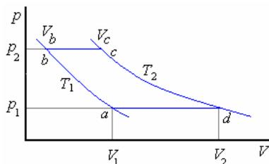
$$b) W_{ab} = nRT_1 \ln \frac{V_b}{V_1} = p_1 V_1 \ln \frac{V_b}{V_1}$$
