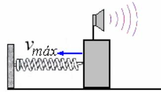
$$f' = f \frac{1}{\left(1 + \frac{v_f}{v}\right)} = 500 \frac{1}{\left(1 + \frac{0,5}{340}\right)} = 499,27 \text{ Hz}$$
