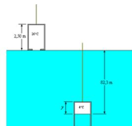
$$\frac{p_1 V_1}{T_1} = \frac{p_2 V_2}{T_2} \Rightarrow V_2 = \frac{p_1 T_2}{p_2 T_1} V_1$$
