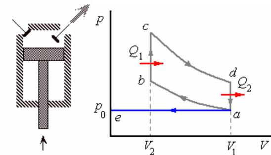
$$Q_1 = \int_{T_b}^{T_c} C_V dT = C_V (T_c - T_b)$$
