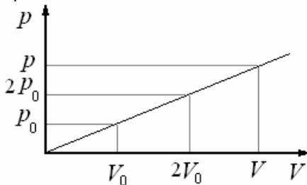
$$\frac{p - p_0}{V - V_0} = \frac{2p_0 - p_0}{2V_0 - V_0} = \frac{p_0}{V_0} \Rightarrow p = \frac{p_0}{V_0} V$$
