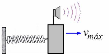
$$f' = f \frac{1}{\left(1 - \frac{v_f}{v}\right)} = 500 \frac{1}{\left(1 - \frac{0,5}{340}\right)} = 500,74 \text{ Hz}$$
